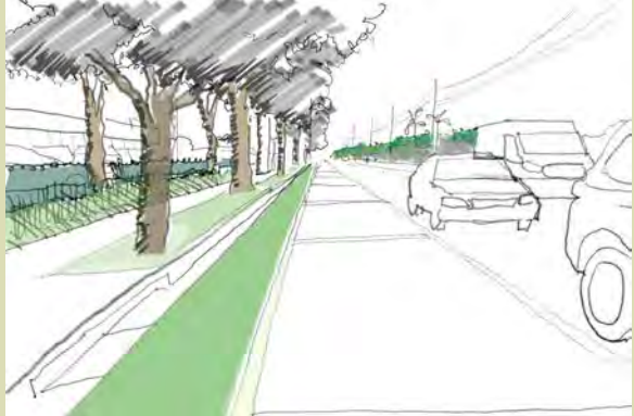
NW 7th Avenue proposed with bike lane curbside and landscaped berms added within ROW to screen parking lots and provide shade for pedestrians.
